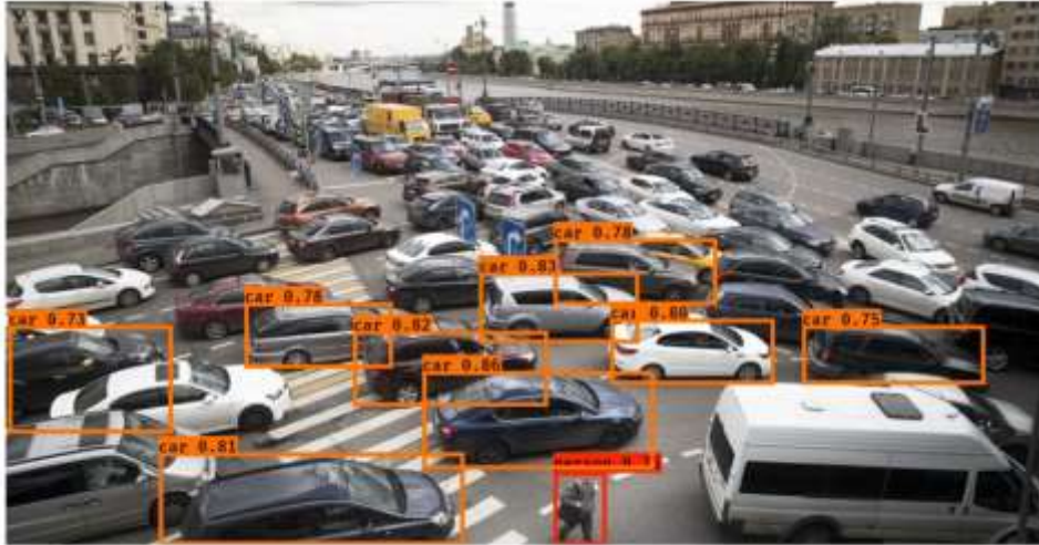
Figure 3.12 YOLOv3 detection with class score (Shivaprasad, 2019).
